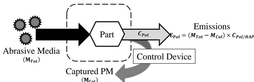
**Figure 7-2. Abrasive Blasting Control Volume – Mass Balance Method**
