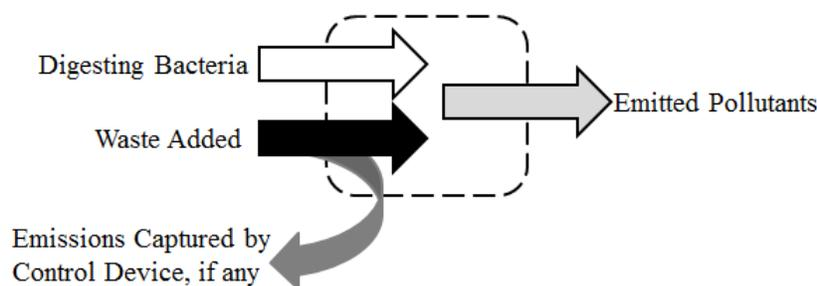
**Figure 15-1. Simplified Control Volume for Emissions from Landfills**
