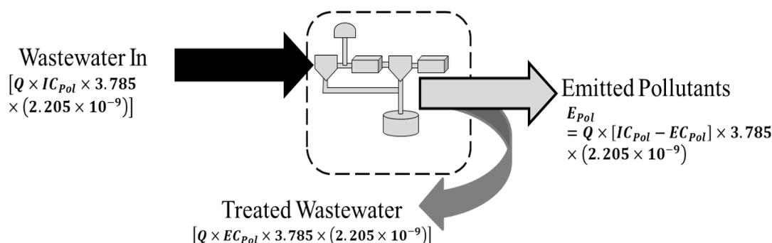
**Figure 23-2. Wastewater Collection and Treatment Control Volume**
