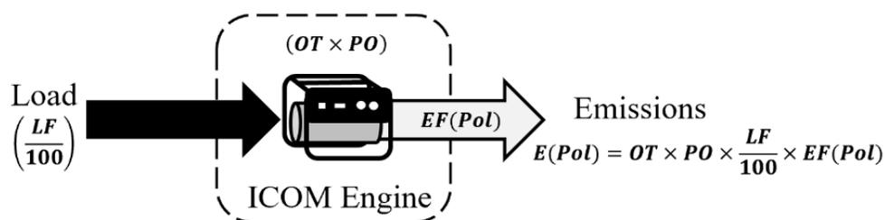
**Figure 3-3. Stationary ICOM Control Volume – Load Factor Method**
