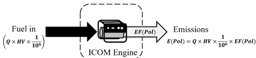
**Figure 3-2. Stationary ICOM Control Volume - Fuel Consumption Method**
