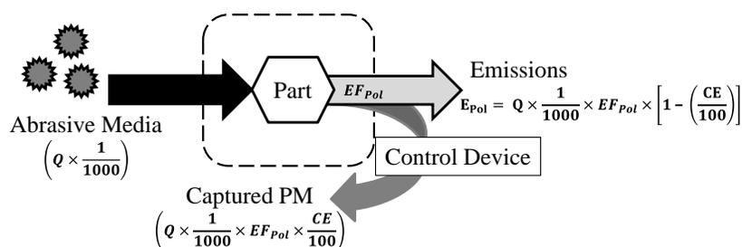
**Figure 7-3. Abrasive Blasting Control Volume – Emission Factor Method**
