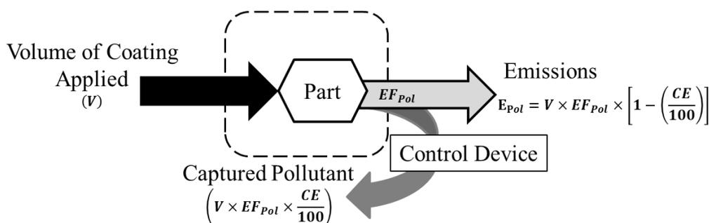
**Figure 22-4. Surface Coatings Control Volume – Emission Factor Method**
