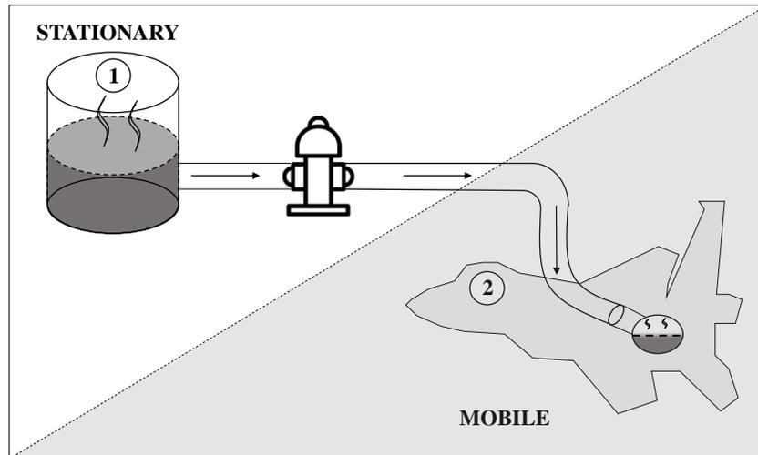
1→2 This figure illustrates fuel transferred to refuel an aircraft from a bulk storage tank via a hydrant system. The vapors displaced within the storage tank as the liquid level lowers or rises are known as “working losses”. Vapors generated in the space above the stored liquid are known as “breathing losses”. These emissions result in **stationary** emissions of pollutants and are calculated in the “Storage Tanks (AST, UST)” section of this guide.
