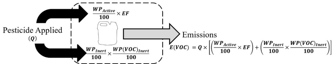
**Figure 18-3. Pesticide Application Control Volume – Emission Factor Method**
