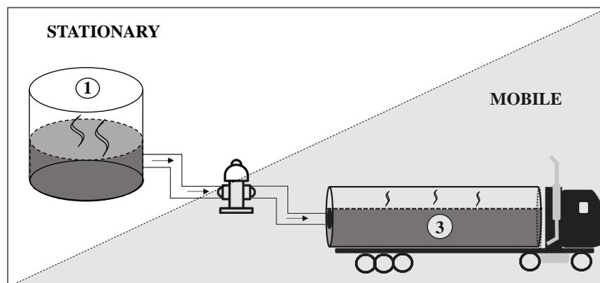
1→3 In this figure, the **stationary** source of emissions is the storage tank producing working losses and breathing losses from the liquid fuel. These emissions, previously calculated by the now incompatible EPA’s TANKS modeling program, can now be calculated with either ACAM or APIMS. This is described in the “Storage Tanks (AST, UST)” section of this guide or with Equation 6-2 if the tank size is below the minimum dimensions required to run the modeling program.
