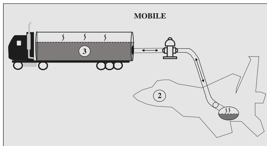
2↔3 This figure illustrates the fueling or defueling of an aircraft via a refueling truck. Both pieces of equipment are **mobile**. All emissions generated from these activities (which come from displaced vapors in the refueling truck or aircraft fuel tanks) should be reported in a mobile AEI and calculated as directed by the *Air Emissions Guide for Air Force Mobile Sources*.
