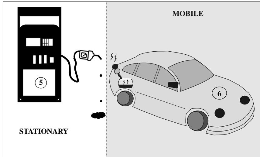
5→6 This figure illustrates the refueling of a vehicle at a service station. The **stationary** emissions are the result of the evaporation of spilled fuel from the fuel nozzle whose calculations are described in Equation 6-3. Another source of stationary emissions come from the working losses of the storage tank as the fuel level is lowered. Therefore, depending on the tank size, the emissions are estimated with ACAM or APIMS, or with Equation 6-2.
