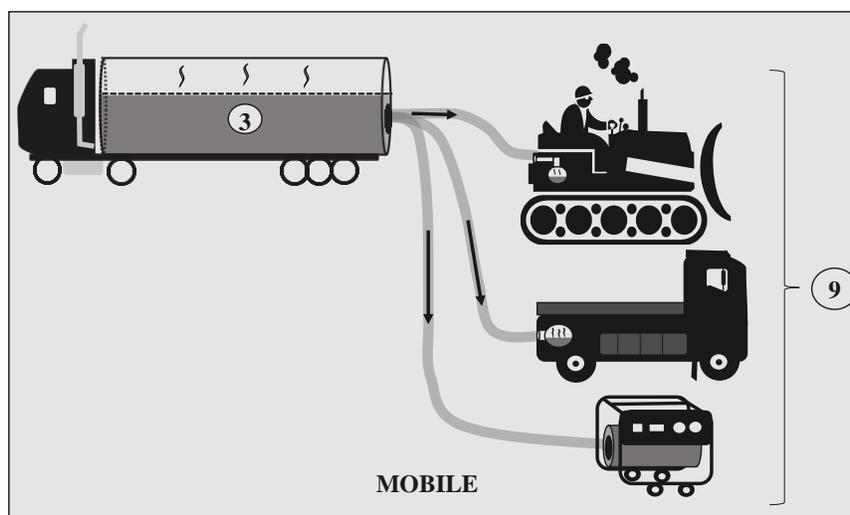
3→9 This figure illustrates the transfer of fuel from a **mobile** fuel loading outlet (refueling truck) into either non-road equipment, GSE, or a mobile generator, **all** of which are considered **mobile** sources. Emissions are calculated as described in the *Air Emissions Guide for Air Force Mobile Sources* and should be reported in a mobile AEI.
